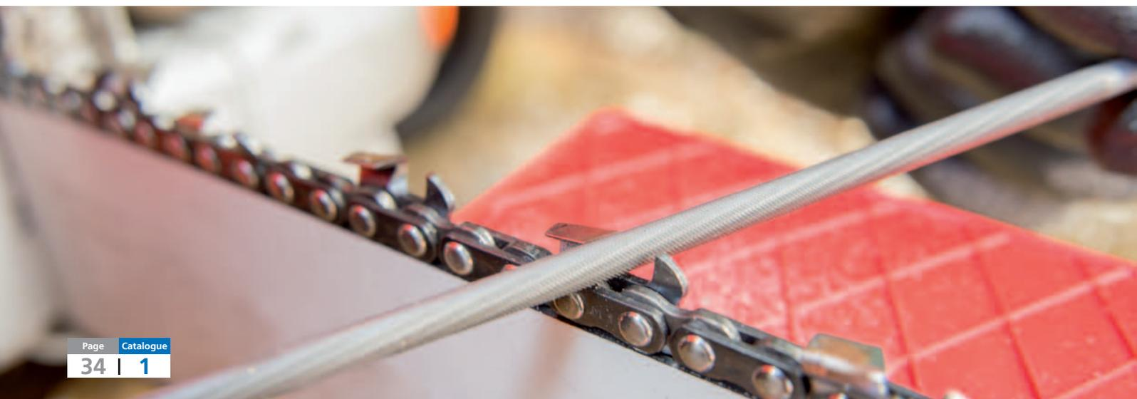
Chain saw sharpeners from PFERD are exceptionally well suited to the manual sharpening of saw chains. Manual sharpening is more economic and much more gentle than machine-based sharpening, and can prolong the operating life of the saw chain.
