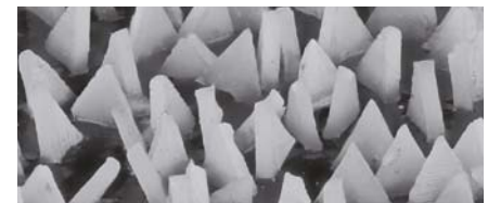
The VICTOGRAIN abrasive grain is optimally aligned
