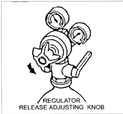
Open cylinder valve and check the cylinder pressure (Must be greater than 10bar (150lb/in 2 )).
