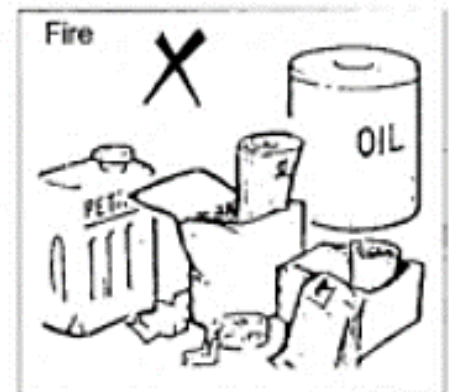
Before commencing welding, clear the area of flammable materials
