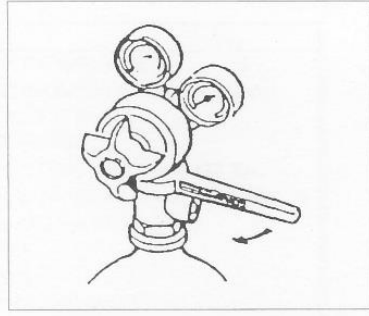
Fit gas regulator to cylinder and hand tighten using correct size spanner. DON'T OVERTIGHTEN 'O' RING, provides seal.
