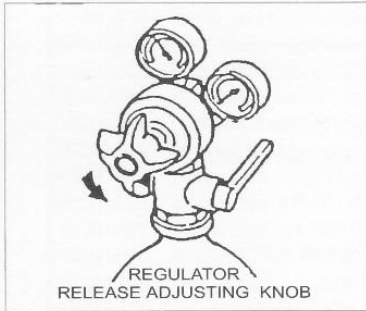
Open cylinder valve and check the cylinder pressure (Must be greater than 10bar (150lb/in 2 )).
