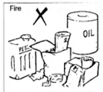
Before commencing welding, clear the area of flammable materials
